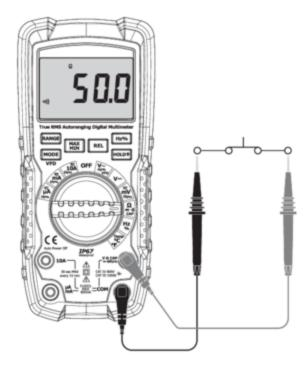
Set the function switch (E) to the Ω → → → ○ CAP position.
